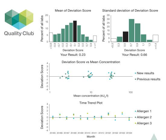
Summary of retrospective results presented using the deviation score's mean and standard deviation. The top panels demonstrate the properties of the preceding year's deviation scores in comparison with deviation scores from all other labs across the world. Ideally, the deviation score should be close to zero and distributed symmetrically around the solid horizontal line in the middle and bottom panel.
